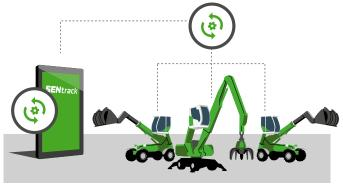
**Software over-the-air:** Long established in the world of smartphones, updates can be loaded directly onto the machine in the G series. This is centrally triggered, so many service deployments can be reduced.
