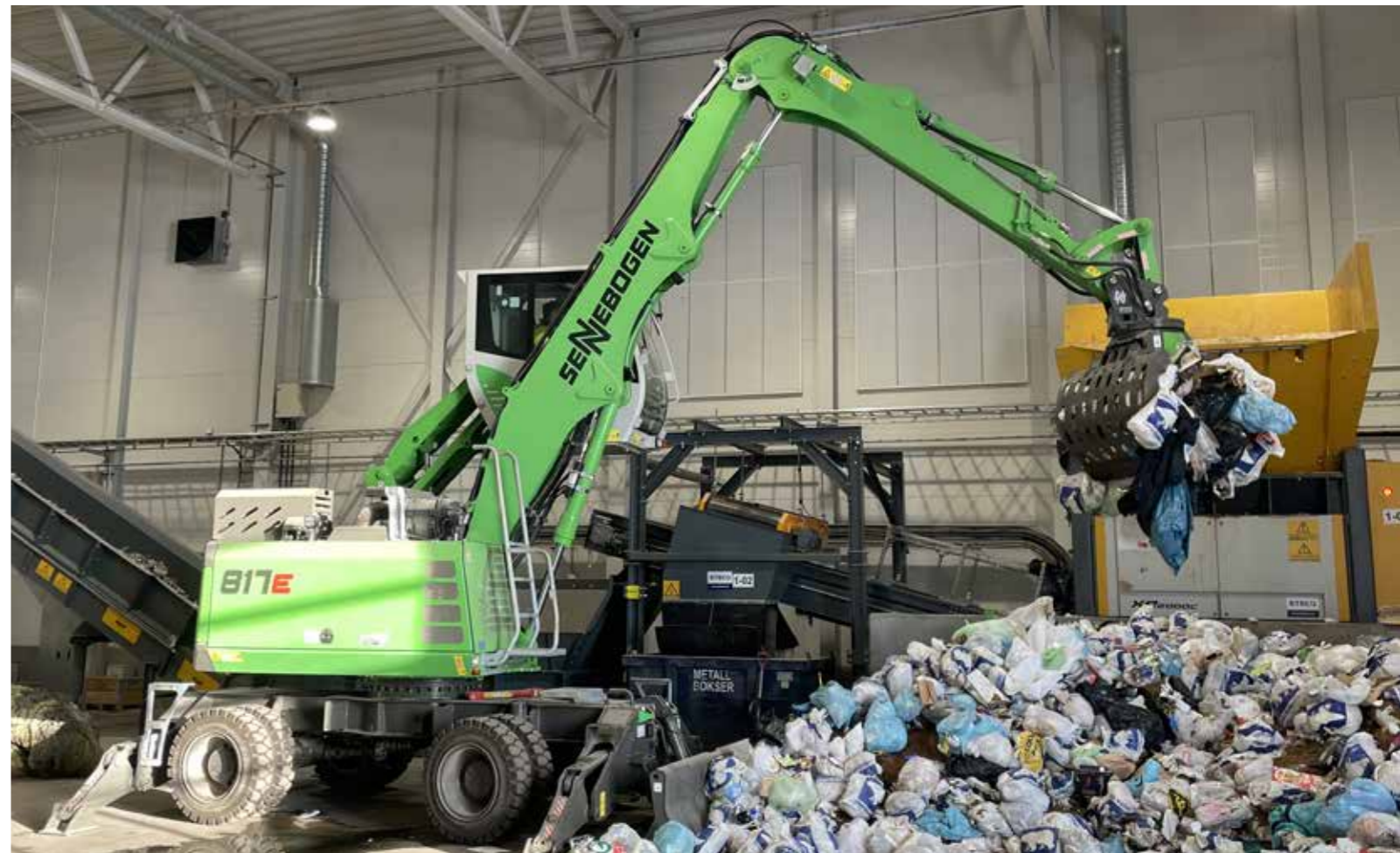
817 M - with sorting grab - loading of shredder indoor; Spitzbergen 817 M - Schredderbeladung in der Halle; Spitzbergen
