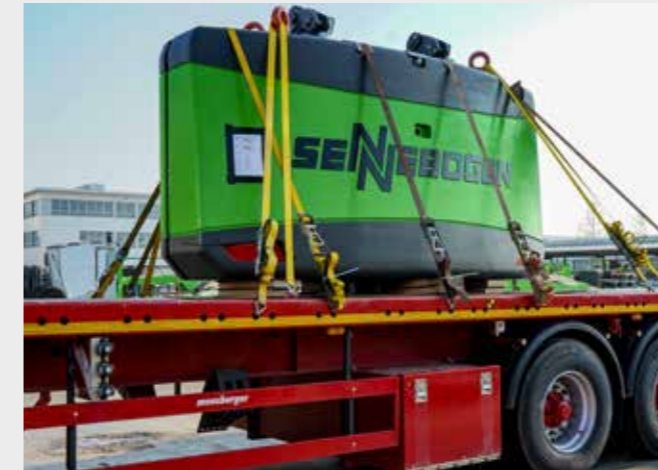
870 Demolition: Removable counterweight reduces transport weight
